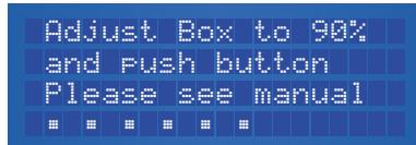
The fan is now running slowly. Rotate the PTB slowly until the fan stops increasing speed. This is the 100% speed. Rotate the PTB back until you feel that the fan is at 90% of its maximum speed.
