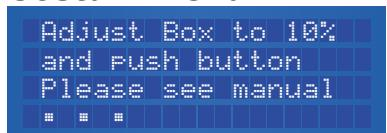
The fan is not running or will run very slow. Rotate the PTB until you feel that the fan is at 10% of its maximum speed. This way, you can decide how much power is needed for 10%.
