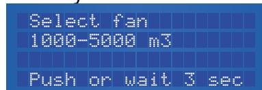
The desired fan can be selected by rotating the PTB. Your selection is set as default after a push on the button. This fan setting will be used when rebooting the Clima Control Plus.
