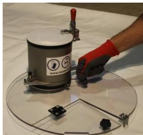
2. Attach the dose mesurer and systematically screw in the screws and ensure that the dose measurer is equally stabilized by the attachments.
