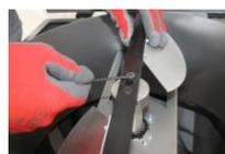
4 Tighten the central screw of the shaft.
