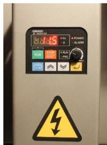
6. The control buttons are the ones at the top (Green and red) and the regulator at the top right hand. The ones on the bottom are only for configuration. Important to read the provided Omron Instructions before use them.
