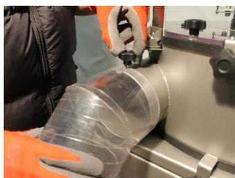
4. Attach the transparent tube in the correct position and use the screw to pin it up.
