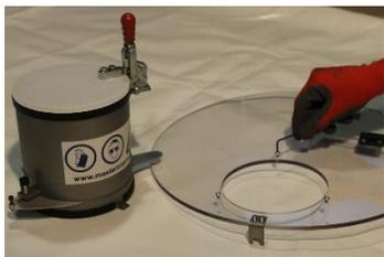
1. With the provided allen wrench remove the screws
