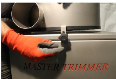
3. Attach the main container on the top of the grid and pin up with the provided screws.
