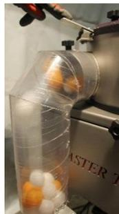
4. Once the desire trim is obtained, increase the intensity to 100% and open the exit door to allow the flowers to fall into the transparent tube.
